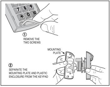
Figure 3. Opening the Keypad
